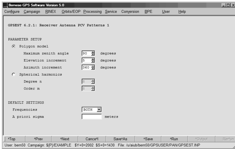
Figure 16.4: Program input panels for the determination of the receiver antenna phase center variation in program GPSEST.
