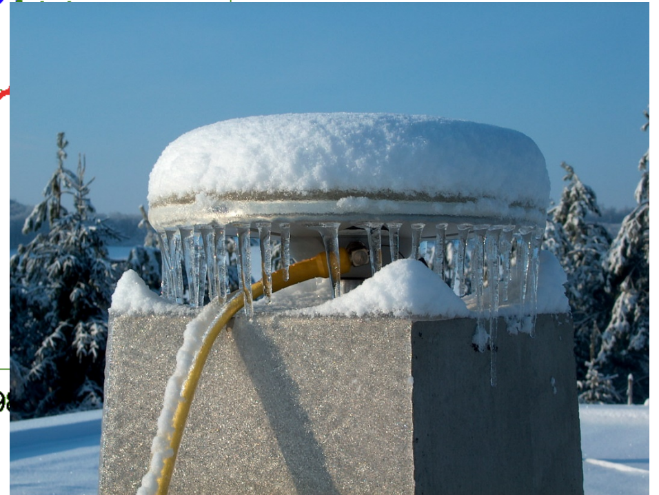
Snow on the GNSS antenna
