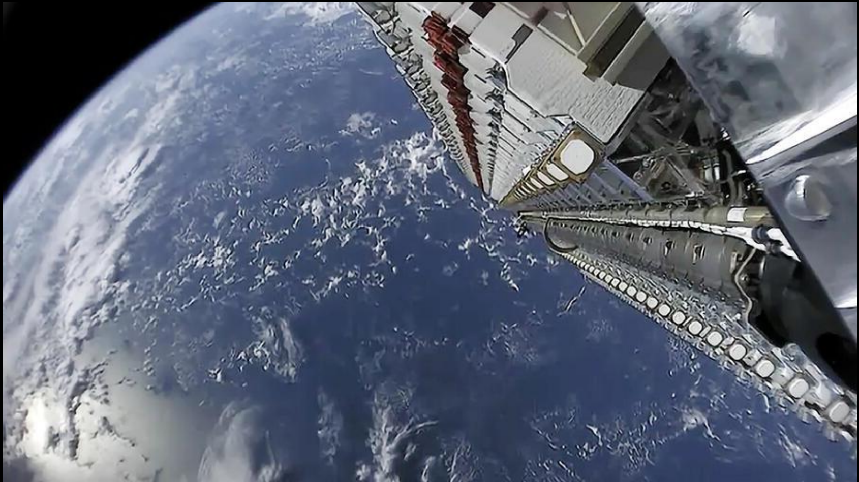
Deployment of Starlink communication satellites from Falcon 9 upper stage
