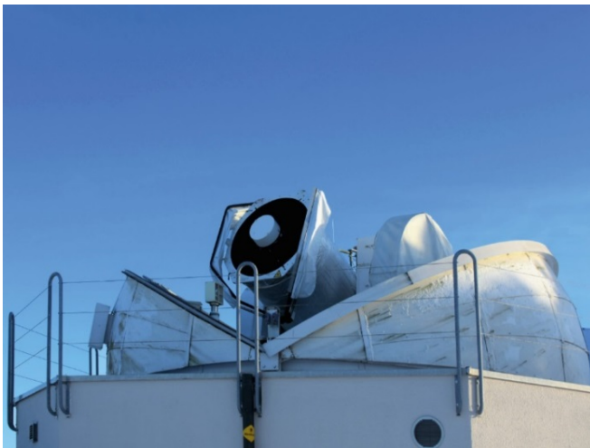
Figure 1: The Zimmerwald Laser and Astrometry telescope ZIMLAT used to range to the space debris object.
